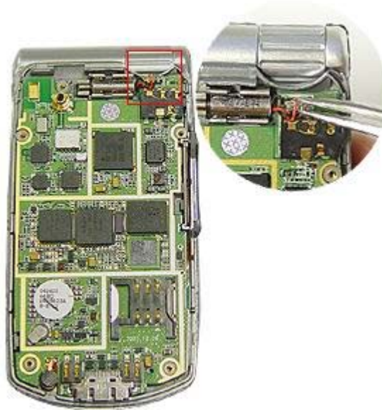
32. Put the metal part (volume control) back to the battery door
