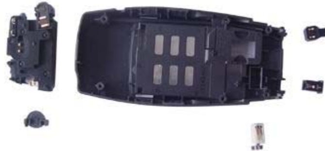
8. Remove the antenna from Nextel 6015i
