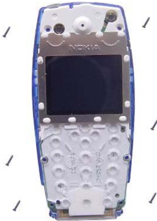
18. Reassemble a new faceplate - Nextel 6015i
