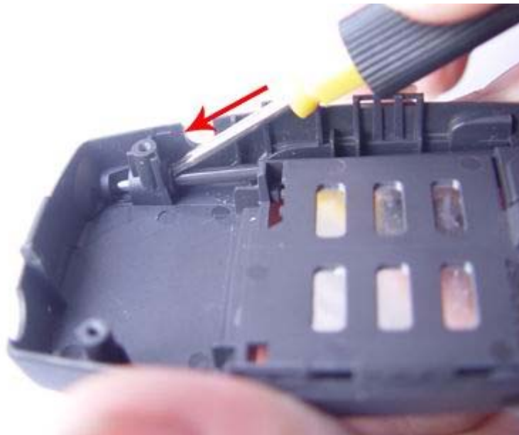
9. Nextel 6015i faceplate installation guide from Accessorygeeks.com
