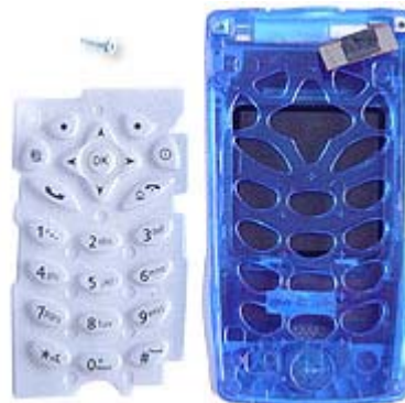
42. Attacg keypad onto the components
