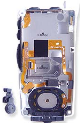
45. Inside view of the battery housing and mid-back
