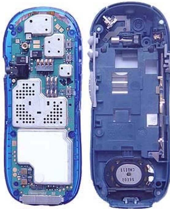
15. Apply all screws and antenna - Nextel i265
