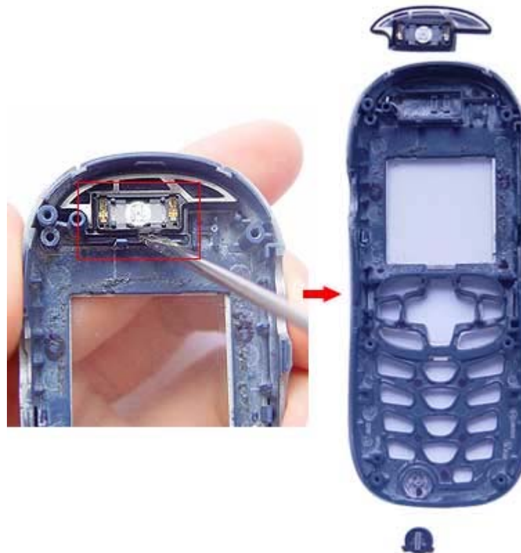
10. Place a camera onto the new faceplate - Nextel i265
