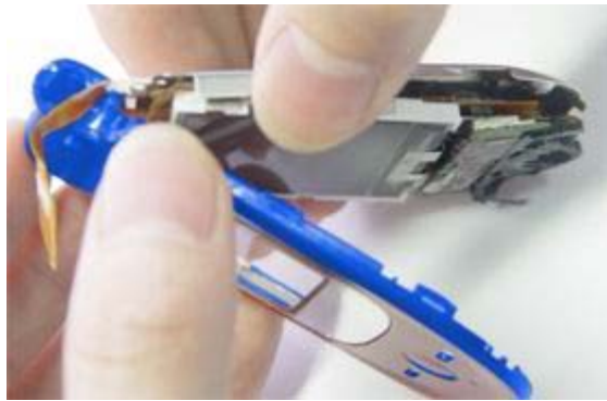
27. Put LCD panel back to the faceplate - Motorola V-220.
