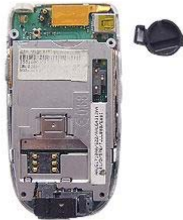
10. Push the yellow tag up from Motorola V-220 faceplate component.
