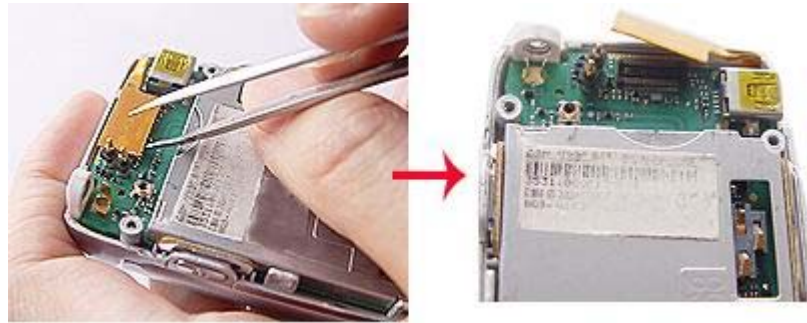
11. Remove metal housing.
