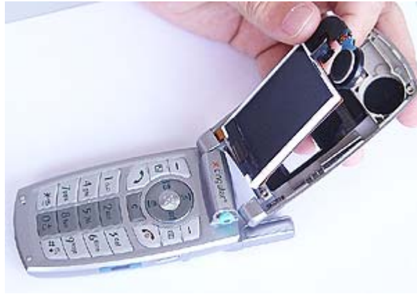
9. LG L1200 faceplate installation guide from Accessorygeeks.com
