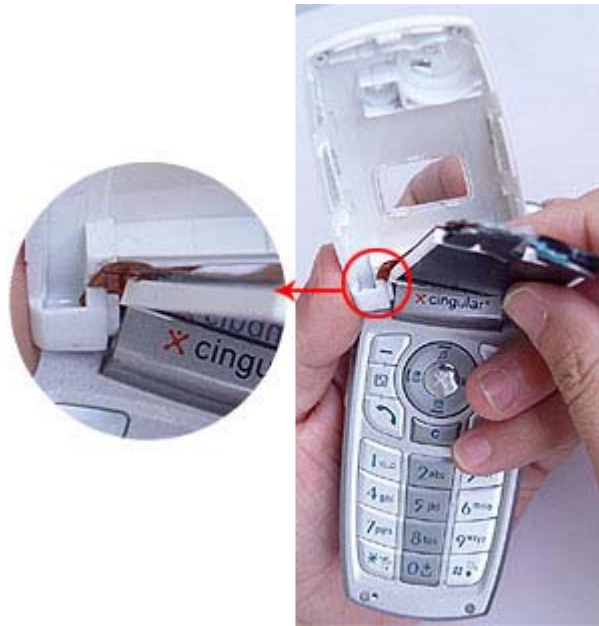
13. Reattach face cover onto LG L1200
