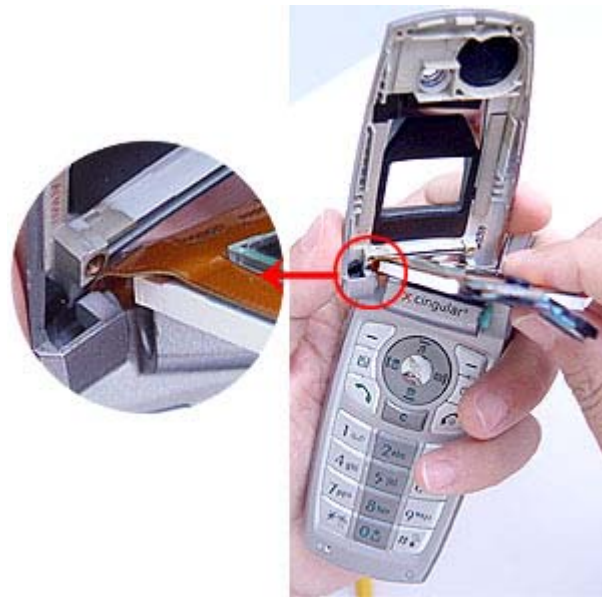
10. Disassemble the face plate - LG L1200
